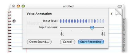
Adjust the input levels. Click "Open Sound" to choose a different input device.
